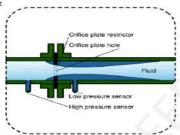
According to Bernoulli's principle, as the velocity of a fluid increases, the pressure it exerts on a surface it passes decreases.
