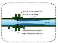
The result is that there is more pressure on the incoming side of the orifice than on the outgoing side.
