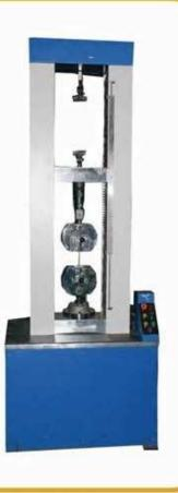
SSS make TNE series machines are electronic screw driven machines with precision screw and column construction and variable speed drive. These are high precision. high performance universal testing machines, maximum capacity up to 200 kN. With the help of computer and micro-computer from control of load to processing of data are carried out with excellent performance, reliability, flexibility and easy operation.
