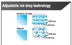
There are three different sizes of ink-drop, users can change the ink drop size to print according to the picture demand level. Make sure the picture has a higher level of accuracy and better sense of depth.
