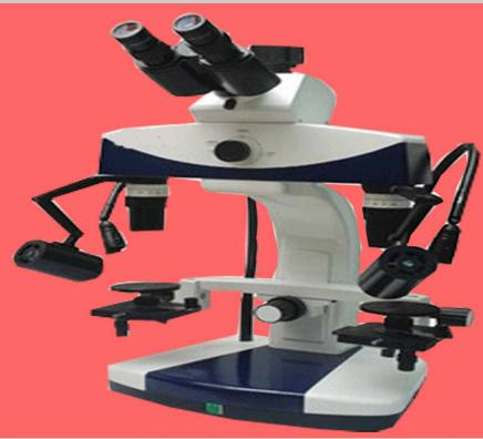
Through optical magnifying, joint and superposition, analyze and compare two images of object field coverage which is observed by the same set of eyepieces to find minimum difference in macroscopy. It's widely applied to distinguish minimum difference, such as bullet, tool mark, fingerprint, character or script and
