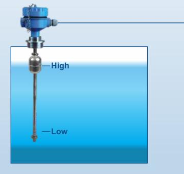
The controller has provision to select pump mode as Pump UP or Pump Down In Pump UP mode, the pump starts at Low Level & Stops at High Level. Pump UP mode is used to Fill the tank.
