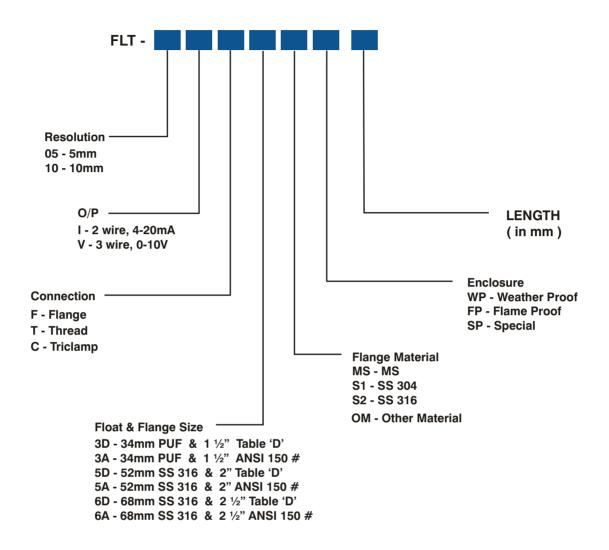
We can also manufacture transmitters with various wetted parts like Polyurethane, PP, PVC, PTFE, etc against specific request.
