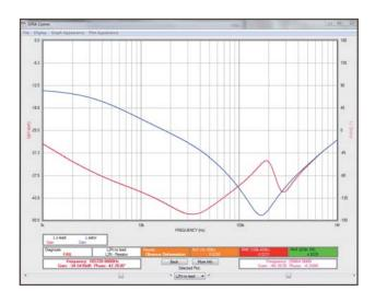
SFRAComm Software provides excellent fault diagnosis assistance, ranging from a sophisticated database including multiple search options to automatic fault diagnosis algorithms in accordance with DLT - 911/2004 and also provides excellent graphing functionality for the more experienced user.
