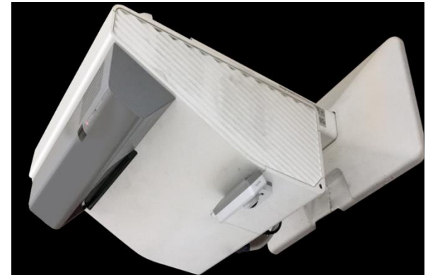
EyeRIS v3.1 attached with normal UST Projector to convert it into interactive projector
