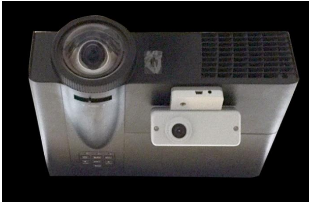
EyeRIS v3.1 attached with normal ST Projector to convert it into interactive projector
