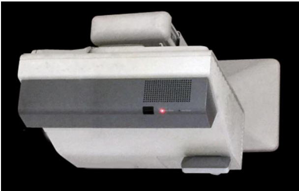
EyeRIS v3.1 attached with normal UST Projector to convert it into interactive projector
