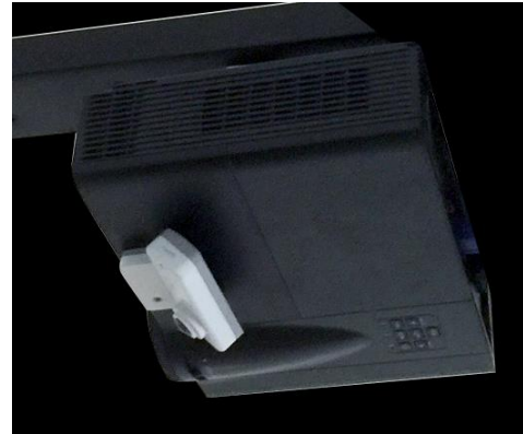
EyeRIS v3.1 attached with normal ST Projector to convert it into interactive projector
