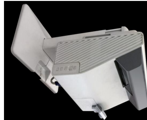
EyeRIS v3.1 attached with normal UST Projector to convert it into interactive projector
