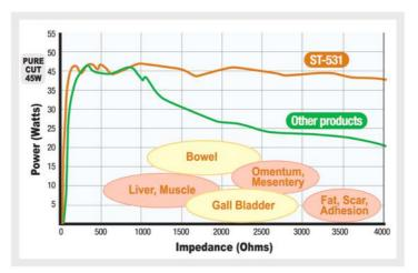
It prevents output power from being reduced over the area where impedance is increased. If impedance is increased over tissue, it produces more output power automatically so it makes it possible to maintain proper output power level during the surgery.
