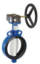
Valves up to size 24" can be direct mounted with gear operators for manual operation. Gear operators can also be attached with chainwheel operators for opening or closing valves located on pipelines at high elevations.
