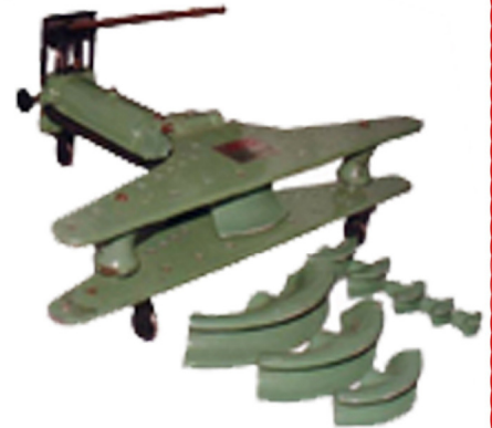
Model:PBM 4 Cap.1.25"-4"(6 Dies) Hyd Hand Operated Pipe bending Machine
