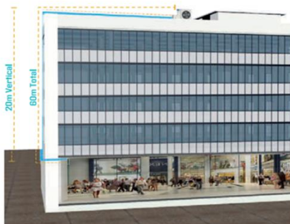
Long Refrigerant Piping
