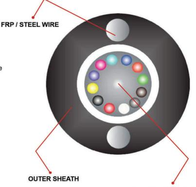
LOOSE TUBE WITH JELLY & FIBRE
