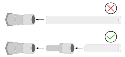
Directly plugging and pulling a teflon hose more than once may lead to particle contamination which can affect the measurement. For this please use the included adapter plugs and keep them on your tubes.
