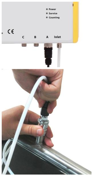
1. Connect the teflon hose with the inlet of the S 130 like shown in the picture.
