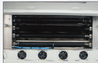
Gumming & Hot Air Drying Unit
