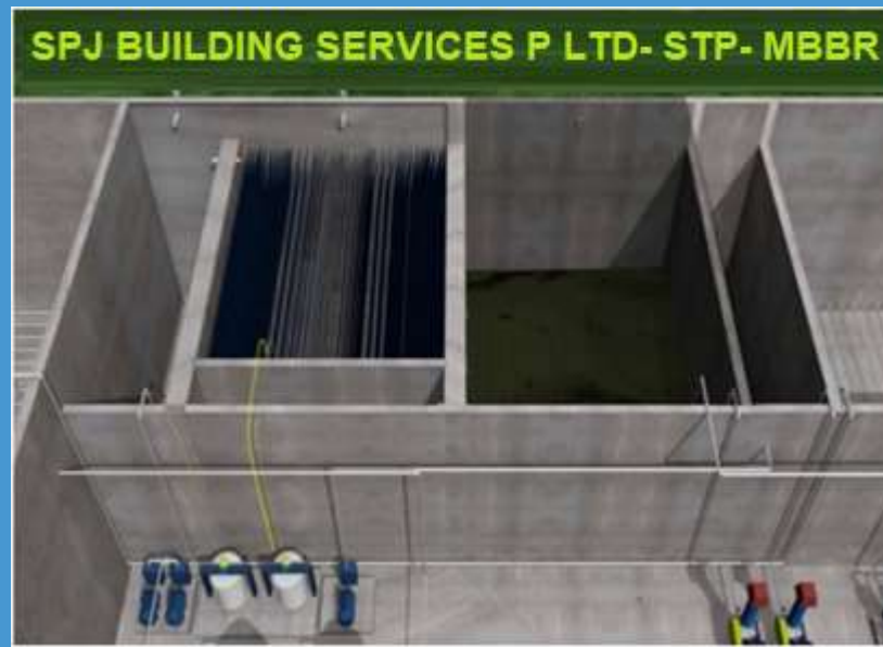
SEWAG TREATMENT PLANT (MBBR)
