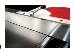
The rip fence can be set as vertical or horizontal way for Support big panel or small work piece.
