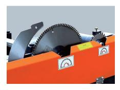
The Splitter can be adjusted as per the main saw blade.
