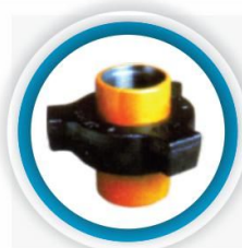
Fig. 602 Black Nut Orange Subs A replaceable lip-type seal ring minimizes fluid flow turbulence and gives pressure seal for air. Water, oil, gas and mud service to 6,000 psi NSCWP*.
