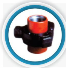
Fig. 400 Black Nut Red Subs Features a precision ball and cone sealing surface for sure metal-to metal seal for air, water, oil, gas and mud service to 4,000 psi NSCWP*.
