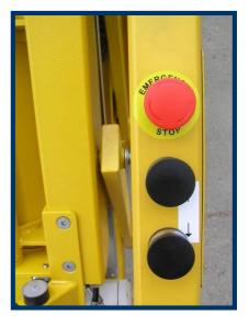
External control buttons are placed on bottom end of travel path. These are used for calling or dispatching platform from or into parking position.
