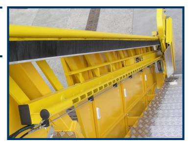
Retainer automatically stop movement of the platform downward in case of breaking load chains or other defect resulting in speed increase beyond limit.
