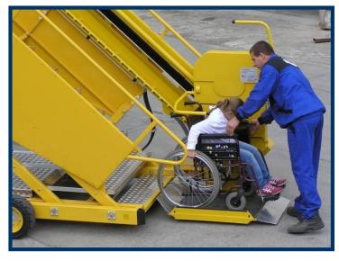
Travel path consists of two beams welded steel profiles, which are hinged to each other. These beams are fixed to the structure of stairs. The slideway for drive chains is part of the top rail. The lower beam is adapted to guide the energy chain with electric cables.
