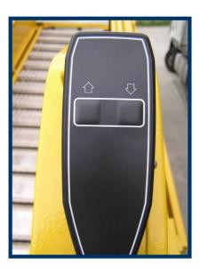
Handheld controller is used to control the platform traveling up and down. It is connected by coiled cable which allows operating from behind or in front of the platform.
