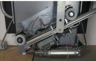
Now bring the platform with the rail to the lower stop position. You can move the rail up and down by using the remote control (drive into and out of carriage) and by this way you can match the rail brackets fix screws on the brackets on the upper side. Then drive up the platform and fix the brackets also in the lower stop area.
