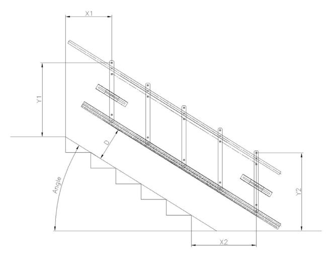
**Step 4:** Adjust the correct angle of the rail. Now check the necessary clearance (dimensions D in illustration) between the lower rail and the step noses. In case the rail angle must be changed to get the correct clearance between rail and step then the angle of the lower platform carriage needs to be changed.
