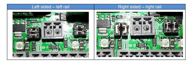
CAUTION: Proper jumper setting is absolutely necessary for the correct and safe function – safety elements in the drive direction.
