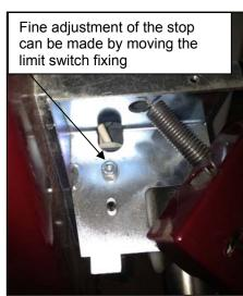
The plastic buffers on the lower end of the backside of the carriage should touch down slightly on the bottom in the **lower stop position**. The lower limit assembly should be placed accordingly!
