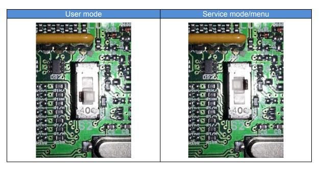
WARNING: After the platform installation and setting all service menu parameters, push the switch S2 to the position for user menu!!!
