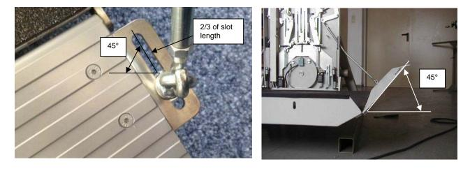
Check the loading ramps for proper operation.
