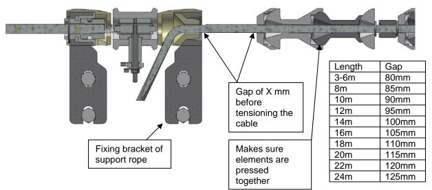
• Below it can be seen how the rope system should look before putting the platform onto the rail.
