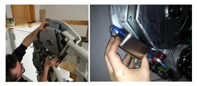
• Remove the over speed governor tube section at the bottom of the system and put the complete rope on the bottom close to the upper motor and make sure it does not get dirty.
