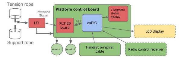
Via the tensions rope the platform is supplied with voltage and information. For the drive commands the user can use a handset or a joystick connected to the platform control. The status of the platform can be seen on the LCD display. A 7.segment display shows the current status of the unit.
