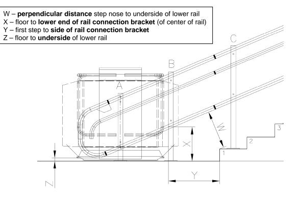
In case of support pillars, these have the serial letters indicated in the drawing that are also stamped on the pillar base plate in order to identify the correct pillar. To facilitate fixing of pillars it helps to provisionally fix the pillars with rope clams.
