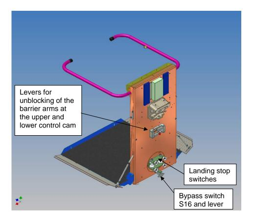
Adjust the position of the control cam in reference to the limit switch device on the rail. The bypass switch has to be activated <u>before</u> the levers for unblocking of the barrier arms touch the control cams on the rail.
