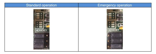
If the jumper J1 was correctly changed then the LD23 should be on. If this is on the platform can be moved. But the drive commands can only be given from the external control (radio or hard wired). At the same time as a drive command is given the button S1 has to be pressed. Both buttons have to be pressed at the same time in order to improve the security during this operation mode. On the display the error 113 will be shown when the platform control buttons are pressed.
