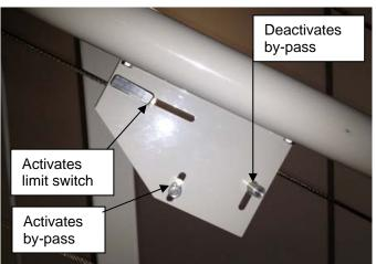
Adjust the ultimate limit switch so that it is properly aligned with the activation pin on the cover of the upper carriage. The pin should reach the switch in case the normal limit switch does not work.
