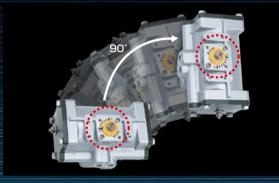
Standard AIR-FAIL-CLOSE mode can be converted to AIR-FAIL-OPEN mode by means of mounting of spring cartridge on the actuator housing reverse end. (spring-return type only) Replacing modular units of blowoff-proof spring cartridge enables accommodation of higher output torque or lower operating pressure. (spring-return type only)
