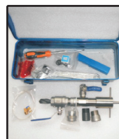
Hot Tapping Driller
