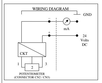
The instrument can be coupled to any reciprocating part to get a direct output of 4-20 mA. The lever of the instrument is fixed to a gear that drives the pinion fixed on the potentiometer shaft. Thus the potentiometer shaft rotates in proportion with the lever which is further connected to the reciprocating part of valve or any other control device using appropriate linkages.
