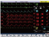
At most 8 channels of waveform display; Various parameter waveforms can be combined and switched freely according to user's demand
